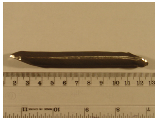
Fig. 1. The digital image of the \text{Ni}_{49.73}\text{Ti}_{50.27} bar which was ECAE processed isothermally at 300^\circ\text{C} with an extrusion rate of 0.25 mm/s.
